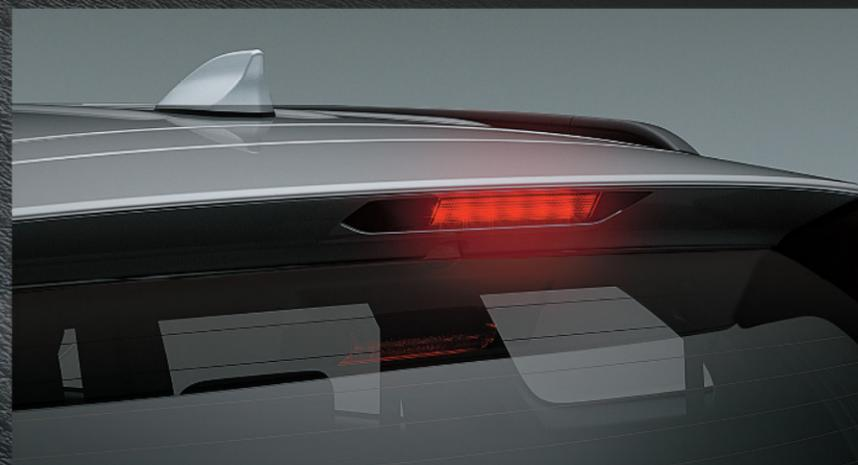
High Mount Stop Lamp with Shark Fin Antenna
